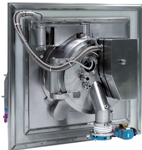
Clean room design, process area side
