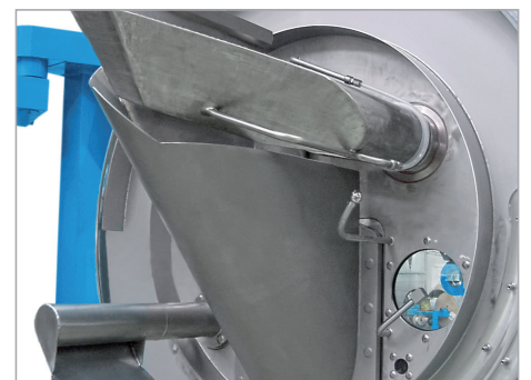
Solids discharge with discharge chute
