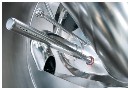
Feed pipe with deflector and wash pipe
