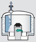
Option 2: Feed pipe and scraper knife over entire basket height with axial movement only Residual heel removal with condensate / sea water
