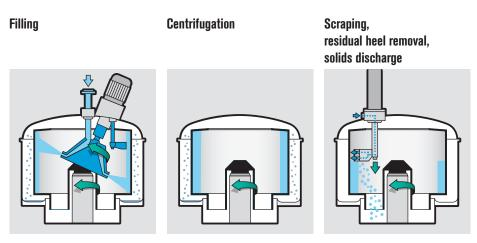
Option 1: Inclined feed disk and scraper knife with axial and vertical movement Residual heel removal during scraping with air / nitrogen
